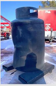
Pictured: Broken weld on old prop due to excessive heat with no cooling of hand lines.
