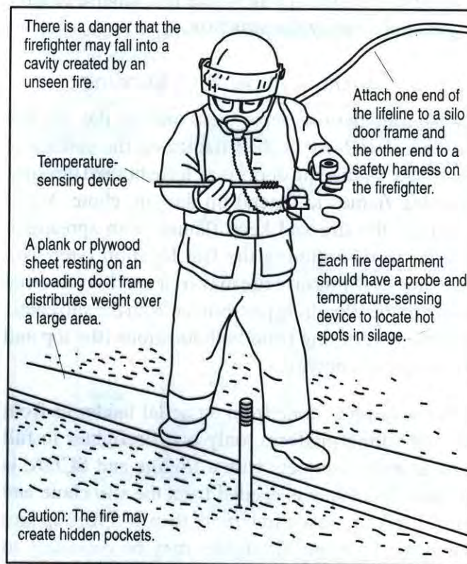
Figure 3-5. Probing for hot spots in silage
