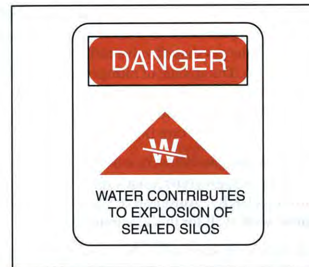
Figure 4-1. Warning sign for oxygen-limiting (sealed) silos Note: These signs are available from D. W. Miller Industries, Inc.; RD #1, Box 7B; Huntingdon, PA 16652.
